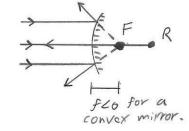
If p>0 and f=0, always true for a convex mirror, then g=0 always for a convex mirror; since (1/p) + (1/g) = (1/f). with g=0, the image for a convex mirror is always virtual.
