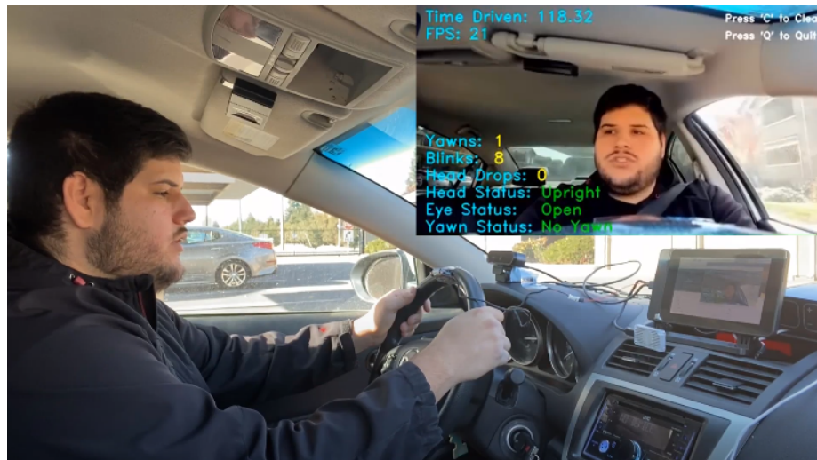
Figure 17. Live Demonstration of the Drowsy Driver Detection System in a Vehicle.
