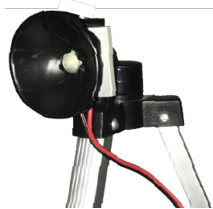
Fig. 11: LED transmitter on a tripod.
