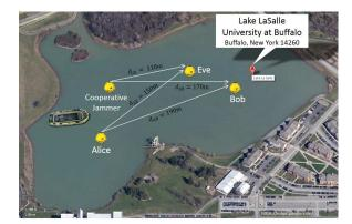
Fig. 7. Aerial view of the underwater acoustic testbed deployment.
