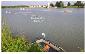
Fig. 6. Actual deployment of the four underwater acoustic modems in Lake LaSalle at the University at Buffalo.
