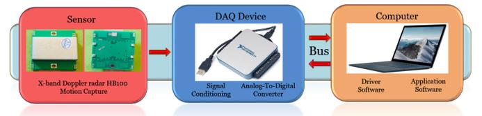
Fig. 1: Interfacing radar sensor with DAQ system.
