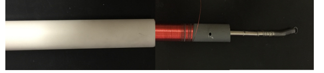
Figure 3: Inside view of the linear electromagnetic generator.
