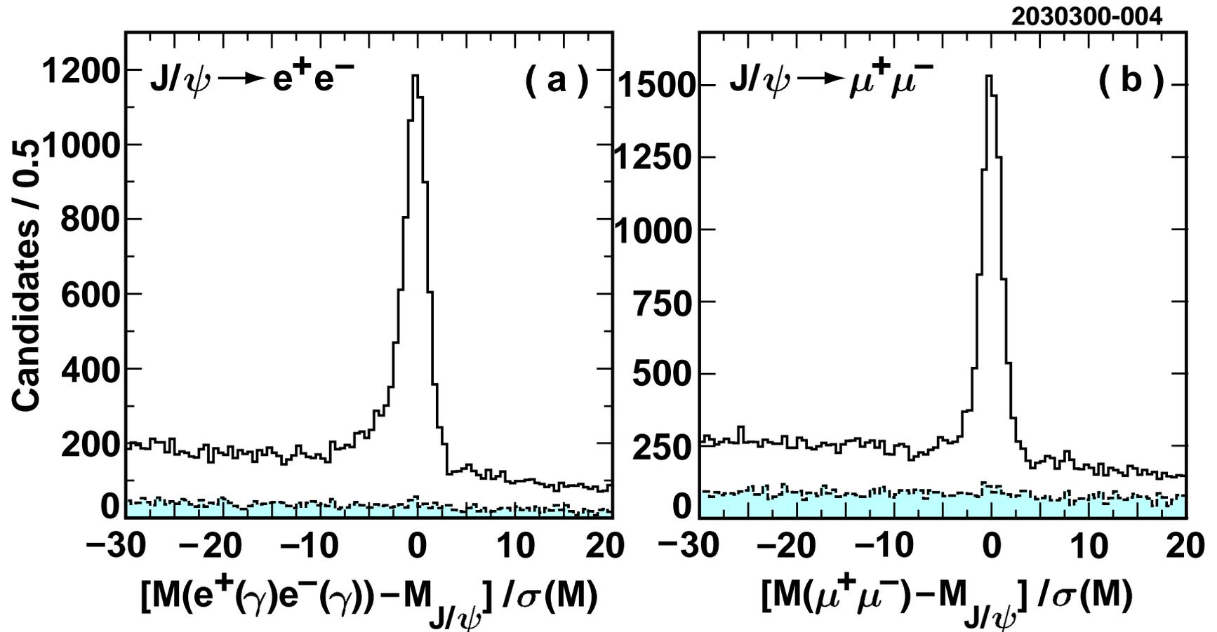
Bremsstrahlung photons from  $J/\psi \rightarrow e^+e^-$  are detected in CsI calorimeter and used in invariant mass calculation
