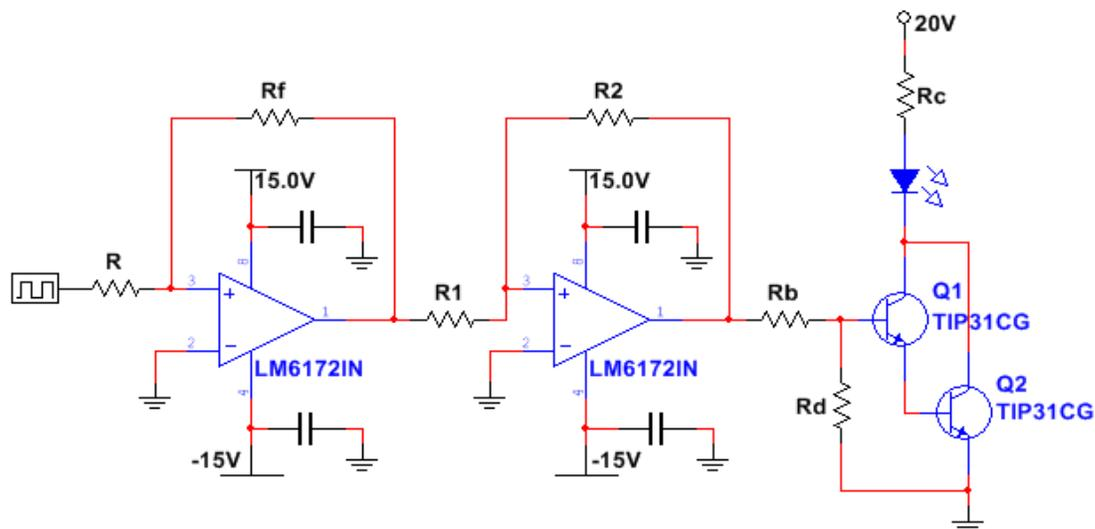
**Figure 3. LED Driver Circuit**
