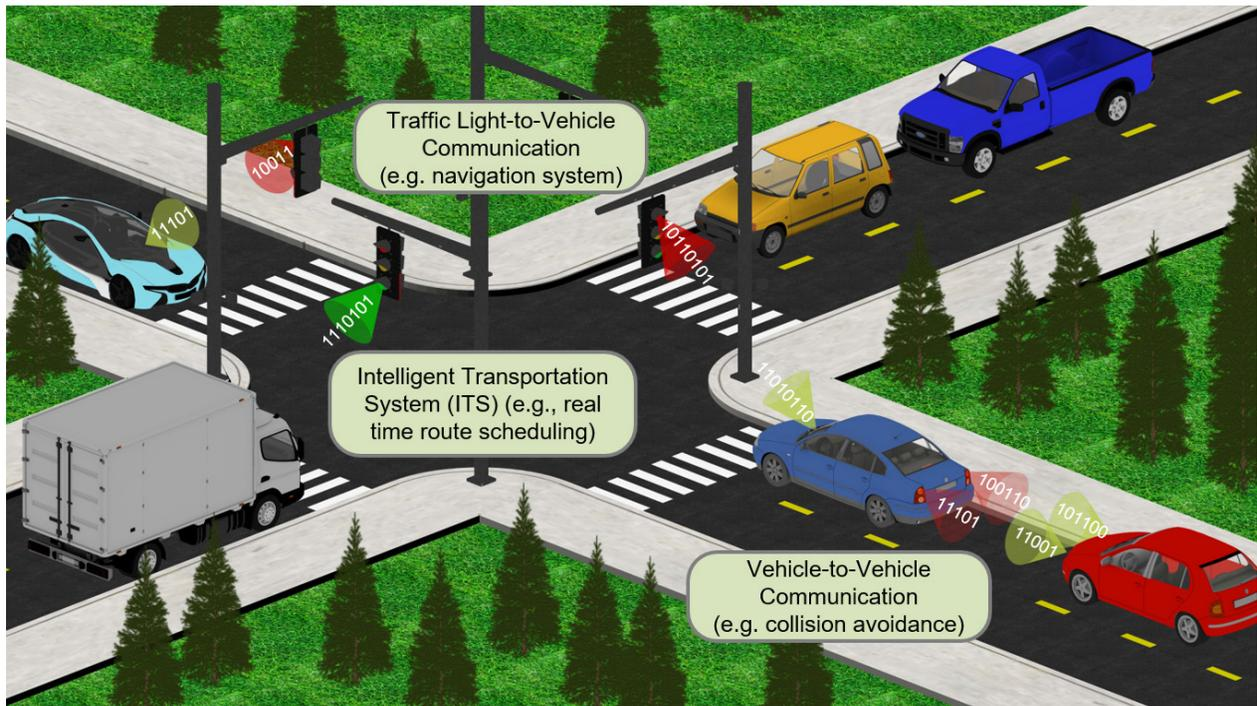
**Figure 1. Intelligent Transportation System Using VLC Framework**
