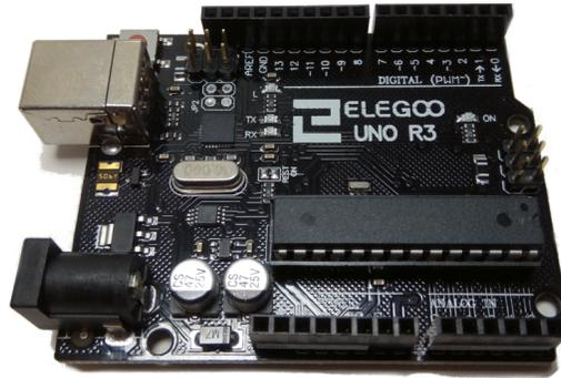
**Figure 18. Arduino Uno R3 Board**
