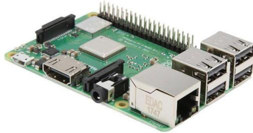
**Figure 12. Raspberry Pi 3 Model B+**
