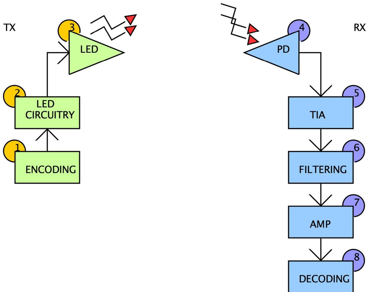
**Figure 2. Block Diagram of VLC System**
