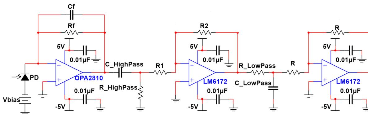
**Figure 4. Photodiode Receiver Circuit**
