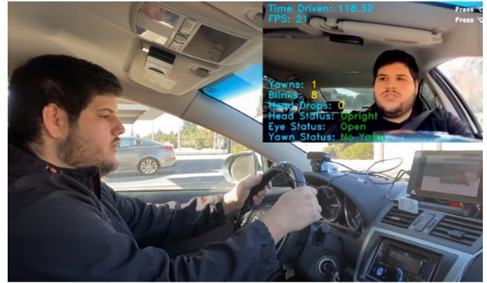
Figure 1. Experimentation of the Drowsy Driver Detection System.
