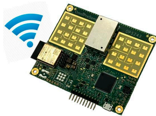
Figure 14. OmiPreSense OPS24-C FMCW Doppler sensor.
