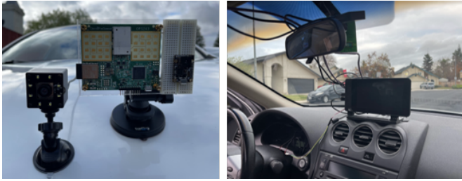
Fig. 9: Pedestrian detection system installed on a vehicle.
