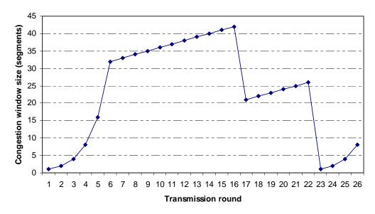
(a) Which TCP protocol was used, TCP-Reno (new protocol) or TCP-Tahoe (old protocol)? Justify using one sentence. (2 points)
